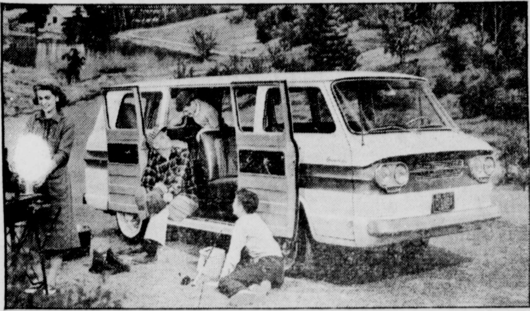
Chevrolet will raise the lid on a real surprise package when they reveal the 1961 Greenbrier Sports Wagon. A promising addition to the Corvair line is this 95-inch wheelbase vehicle with rear-installed engine and independent suspension. The Greenbrier is certain to fit transportation needs from backwoods camps to swank hotels. Seats may be repositioned to fit specialized requirements. There also is a commercial counterpart—a delivery vehicle named the Corvan.
