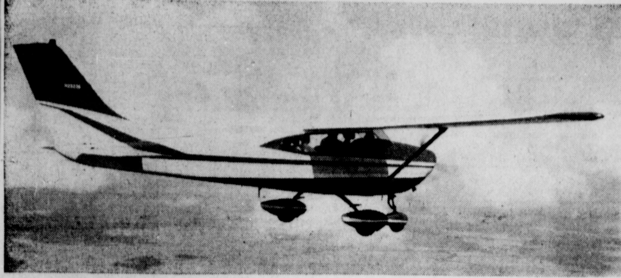
The new swept fin and rudder on Cessna's 1960 Skylane emphasize the graceful lines of the airplane and its complete new exterior styling. Over 1,350 Skylanes have been sold since the airplane was first introduced in 1958. Virgil Rhodes, who owns and operates Hi-Plains Aviation at Abernathy Airport, is a dealer for the 1960 line of Cessna airplanes.
