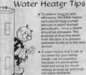
★ To assure long life and efficiency, the water heater tank should have a small amount of water drained periodically. Once a month should be adequate. The purpose of draining water from the tank is to prevent sediment build-up in the tank
