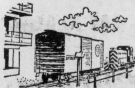
1 Cars from incoming freight trains are uncoupled and nudged one at a time over the crest of a small artificial hill, called the "hump."
