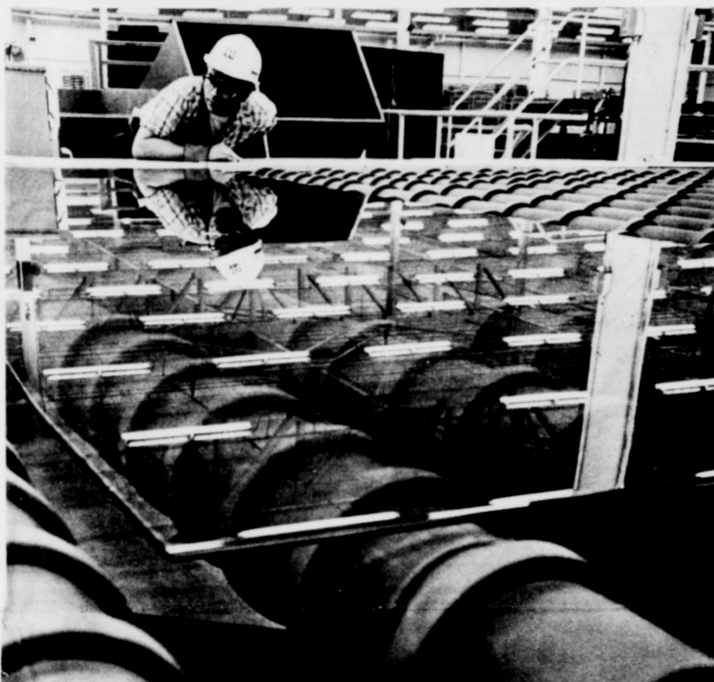
ROLLING REFLECTIONS identify the all-but-invisible float glass panels produced at PPG Industries' big Carlisle, Pa., plant. PPG has announced plans for an even bigger operation near Wichita Falls. Expected to be the world's largest float glass facility, the Wichita Falls plant will have a production potential of more than 400 million square feet of float glass yearly, primarily for the construction and transportation industries.
