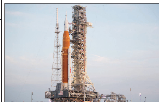
Courtesy photo NASA's Space Launch System (SLS) rocket with the Orion spacecraft aboard is seen atop the mobile launcher as it is rolled up the ramp at Launch Pad 39B Wednesday.
