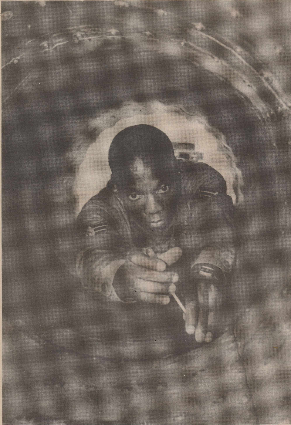
Senior Airman John E. Pruitt removes a firewall panel in a T-38 Boattail. He was promoted to Senior Airman Below the Zone in July. He is assigned to the 64th Organizational Maintenance Squadron.
