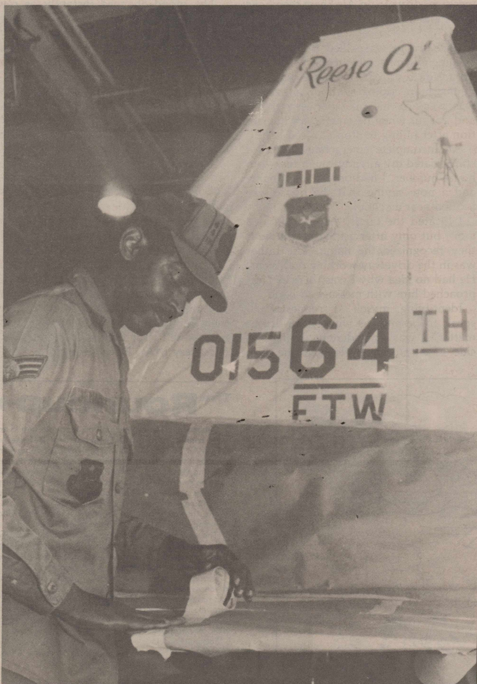
Senior Airman Charles Jennings tapes down over-spray covering on the 01 T-38 before re-painting the nose and the new wing commander's name. The Philadelphia, Pa. native is assigned to the 64th Field Maintenance Squadron Corrosion Control Branch.
