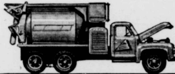
NOW 1 TON MORE GVW —Ford T-800 tandem now has 42,000 lbs. GVW. 170-h.p. Short Stroke V-8. 11,000-lb. front axle available. Increased capacities also apply to corresponding Cab Forward models.
