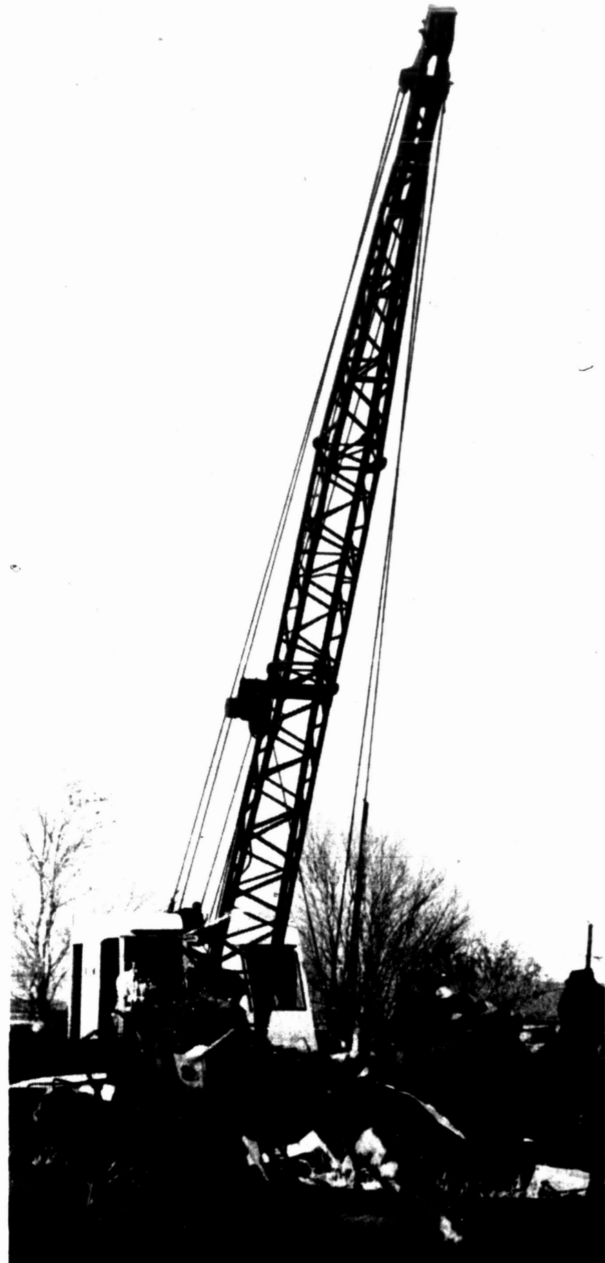
BIG LOAD — Snyder Iron and Metal received this electromagnet crane recently, enabling employees to load scrap steel and iron in as little as three hours per truck load, or about 30,000 pounds. According to crane operator Chris Maxfield, the electromagnet is capable of lifting 6,000 pounds of prepared iron at a time. (Howard Bigham Photo)
