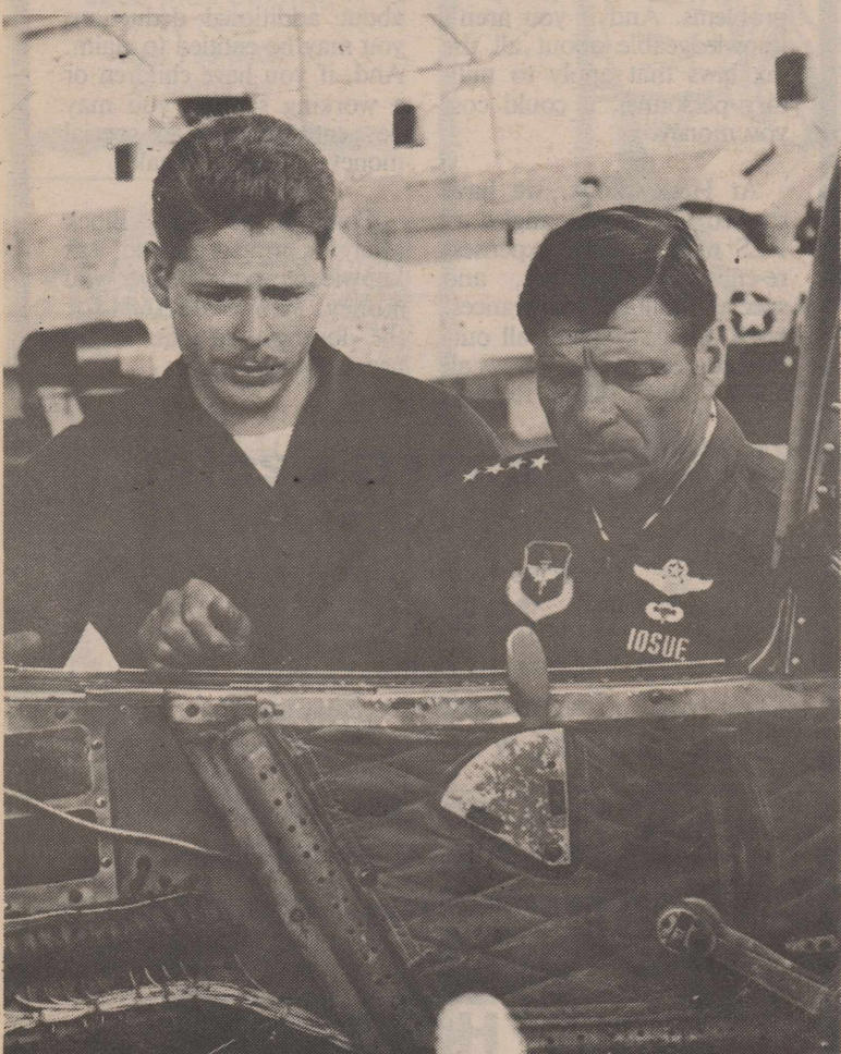
SSgt. Mark Christian points out specific sealing improvements to reduce smoke in the T-37 cockpit.
