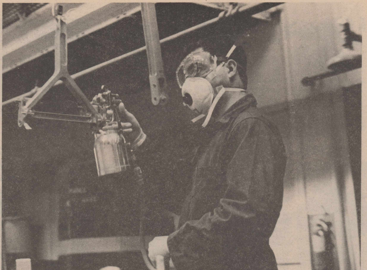
A1C David W. Crosby of the Corrosion Control Branch of FMS primes a drag brace from a T-37. He has been assigned to Reese AFB for two years. USAF Photos
