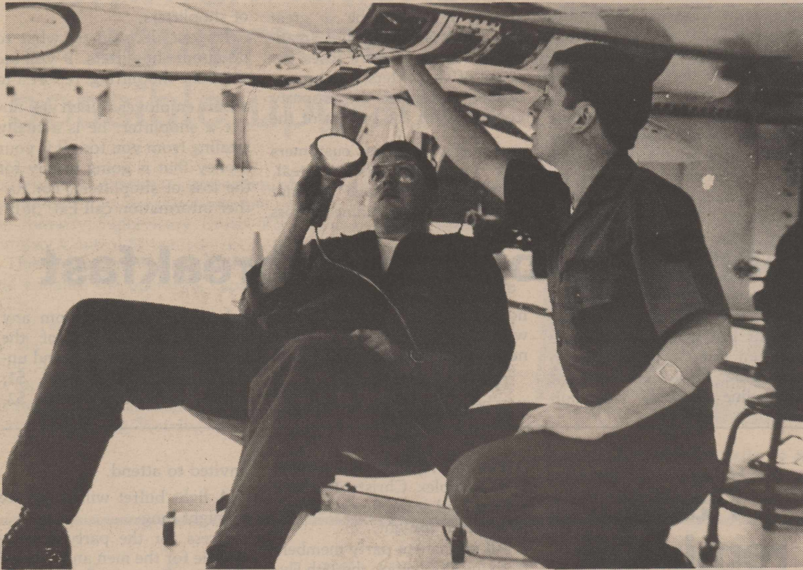
A1C Kent Miller (left) observes as SSgt. 'Doc' Holiday checks flight control cables on a T-38.
