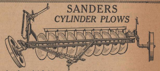
Large Capacity. Light Draft. A general purpose plow. Ideal for Summer plowing but equally good in Cotton, Corn and Maize in the Fall. Plows 2 to 6 inches deep. Easily adjusted and operated. Turns the soil over. Leaves the surface thoroughly harrowed and without ridges.
