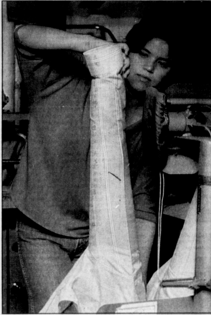
Cruz Carrasco uses a "sleever" to remove wrinkles from shirt sleeves. The rest of the shirt is then finished on a regular press.
