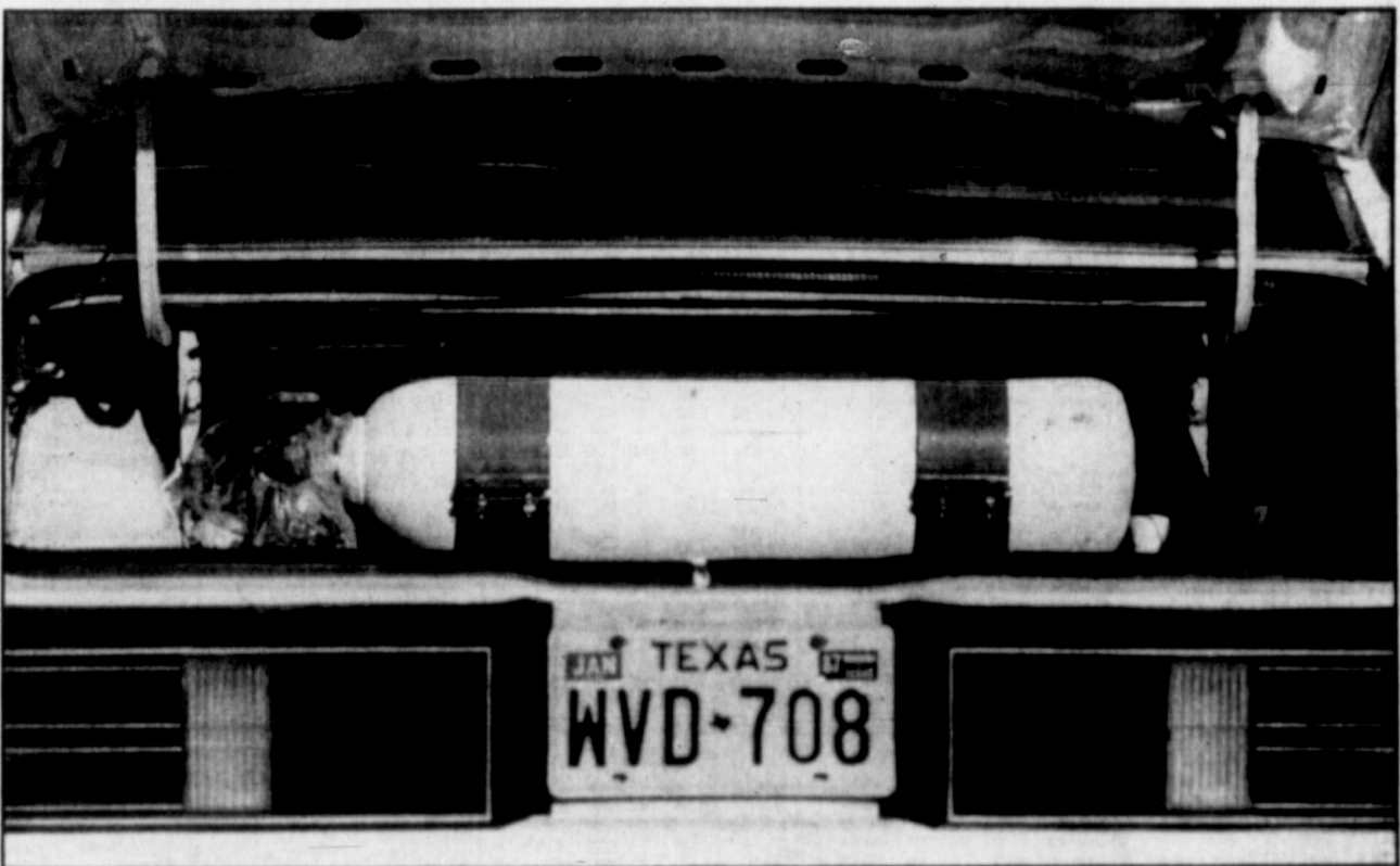
Small tanks such as this may be standard equipment on automobiles in the future if a push to market compressed natural gas is successful.
