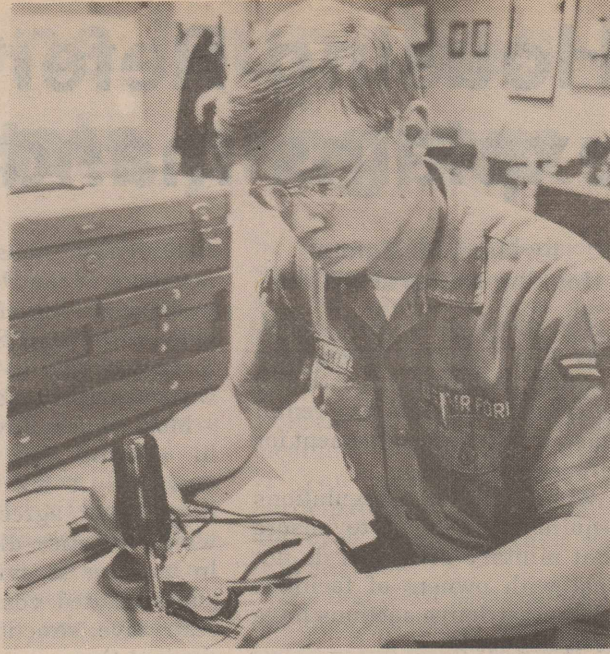
Delicate touch A1C Brett McIntire shows a delicate touch while soldering a transistor checker in the Nav-Aid branch.
