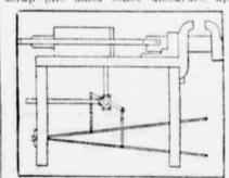
old vise, A, in which the screw had, of the race, become nearly worn out, was connected to the air brake cylinder, B, in such a way that the air entering the cylinder brought the jaws of the vise together. When the air was re-
