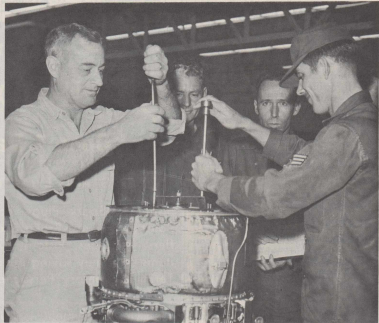
LABOR CHECK—A management engineer, MSgt. Alton Utsey, second from right, checks efficiency in compressing a No. 3 engine bearing for airseal runoff on a T-85 engine used by the T-38 jet trainer. Workers in the base engine shop, left to right, are Randall Madison, mechanic; E. G. Brown, quality control inspector; and A1C Leon Harrell, crew chief.
