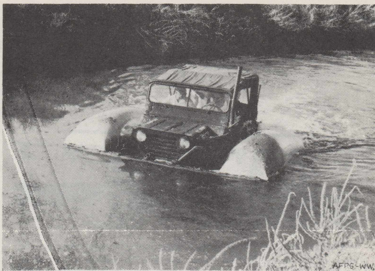
AMPHIBIOUS QUARTER-TON—The driver of this vehicle becomes a pilot when the water wings are used for floating along in deep water. Rubberized nylon bags are inflated with exhaust gases from its motor and the floating vehicle is propelled by the action of its wheels in the water. This new type swimmer is being tested for possible military use.
