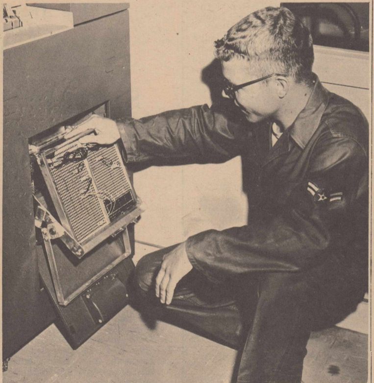
NOT SO EASY — A2C Richard T. Hall, data processing machine operator, arranges a wiring sequence on a control panel which will 'tell' an IBM collator what to do. A different wiring sequence is required for every operation.
