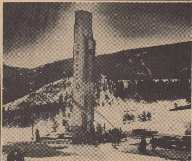
ON DUTY —Technicians supervise the loading of an Air Force solid-fuel Minuteman ICBM from its transport-erector into an underground launch pad at Malmstrom AFB, Mont. Two flights of 10 missiles each are operational with SAC. The first flight of missiles was ready to go before the Cuban crisis.
