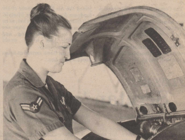
KEEP IT CLEAN! 64th Organizational Maintenance Squadron aircraft maintenance specialist A1C Pam Day cleans a Cessna T-37 Tweety Bird's air conditioning system to prevent foreign object damage (FOD). She has been working on Tweets at Reese for 10 months. (U.S. Air Force Photo by Maj. Joseph Whitaker)
