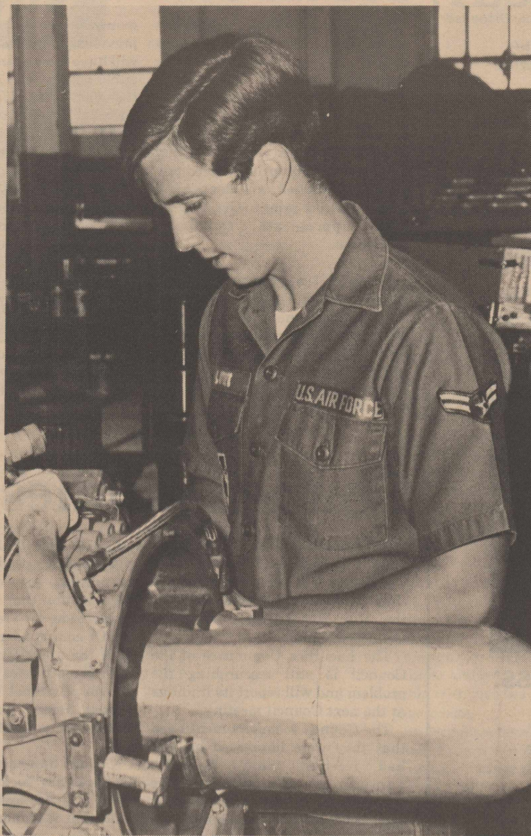
ENGINE REPAIR - A1C Gary Lowe performs maintenance work on one of the J-69 engines that come into the 64th Field Maintenance Squadron for repair. Airman Lowe was named Airman of the Month for June. (U.S. Air Force Photo By Sgt. Terry Crooks)
