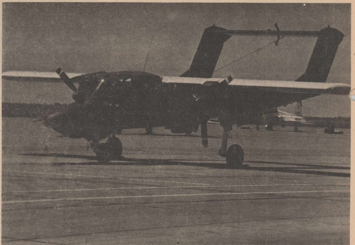
WHAT IS IT?—This somewhat strange looking aircraft pulled up on the flight line recently during a stop on a cross-country mission. It is a North American OV-10 Bronco. It is a two-man, twin-engine, lightly armed reconnaissance aircraft. (U.S. Air Force Photo by Sgt. Dennis Mehrenberg)
