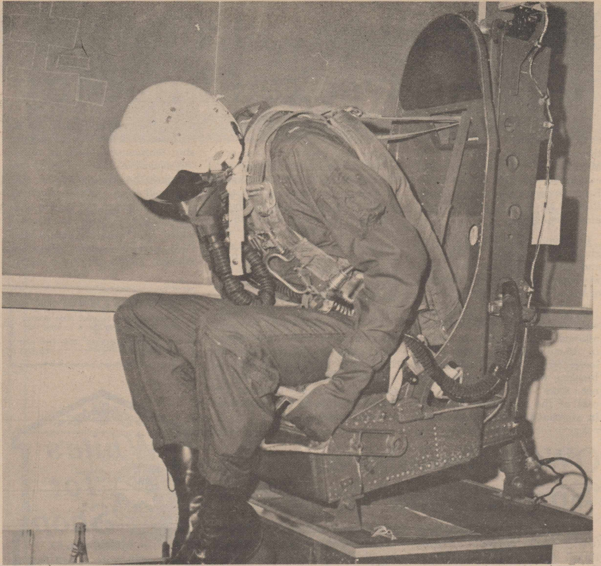
EJECTION PRIMER —Students learn how the ejection seat works in a specially designed simulator. When activated, the seat disconnects all attached hoses as it dumps the student forward, freeing him.
