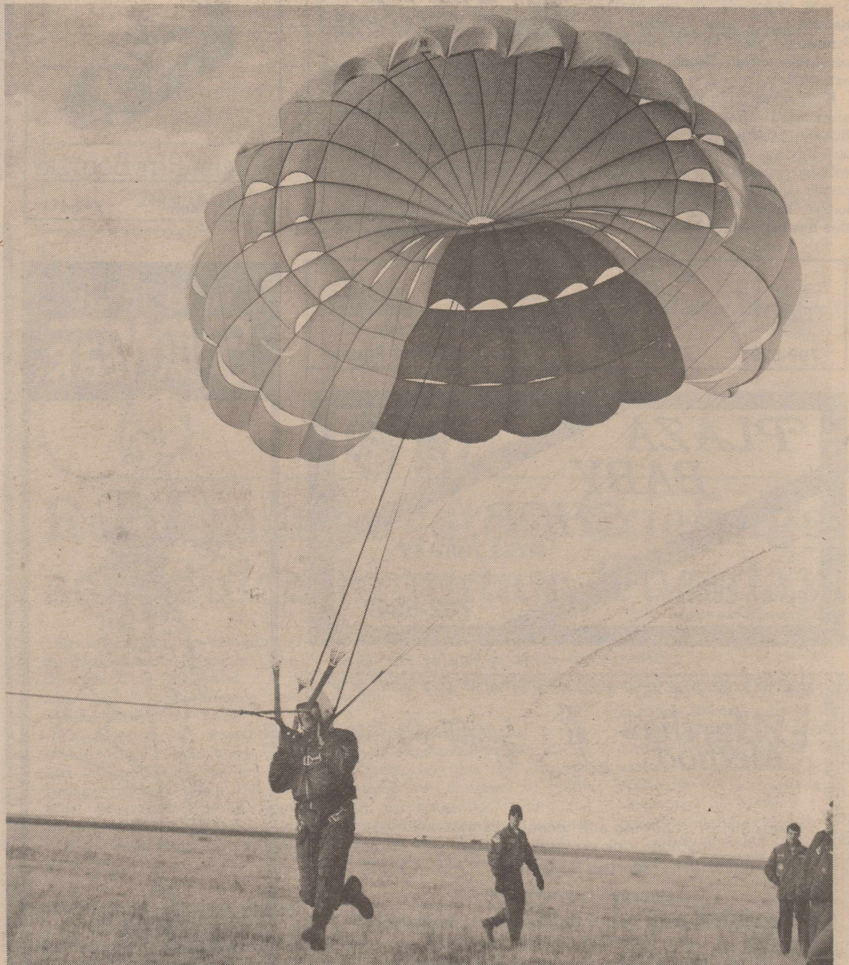
UP WE GO —Parasailing teaches student pilots the techniques of controlling a parachute and landing. Trainees are hooked to a parachute with a harness and a pickup truck via a 900-foot rope. After a few quick steps they become airborne.
