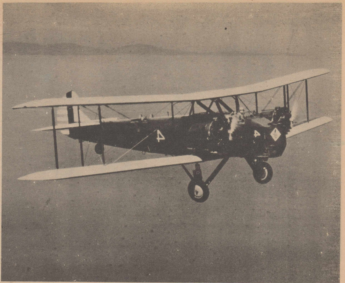
HISTORICAL AIRCRAFT —The Keystone B-3, first of the "B" category bombers. Delivered to the newly established Army Air Corps, it had a 74-foot 8-inch wingspan and a gross weight of more than 12,950 pounds. The B-3 was powered by two 525 horsepower, air-cooled radial engines and had a crew of five.
