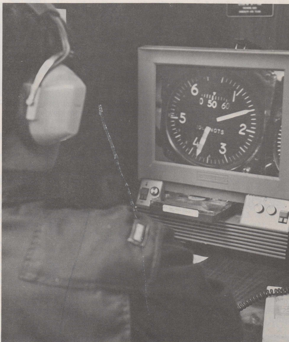
LEARNING CENTER —A UPT student studies instrument procedures in a study carrel of the 3501st PTS Learning Center using a film cassette inserted in a rear-screen projector. The center, which opens today, features 50 of the super 8mm films which allow the student to "visually fly" the mission while receiving authentic instructions through ear-phones he wears. (U. S. Air Force Photo)
