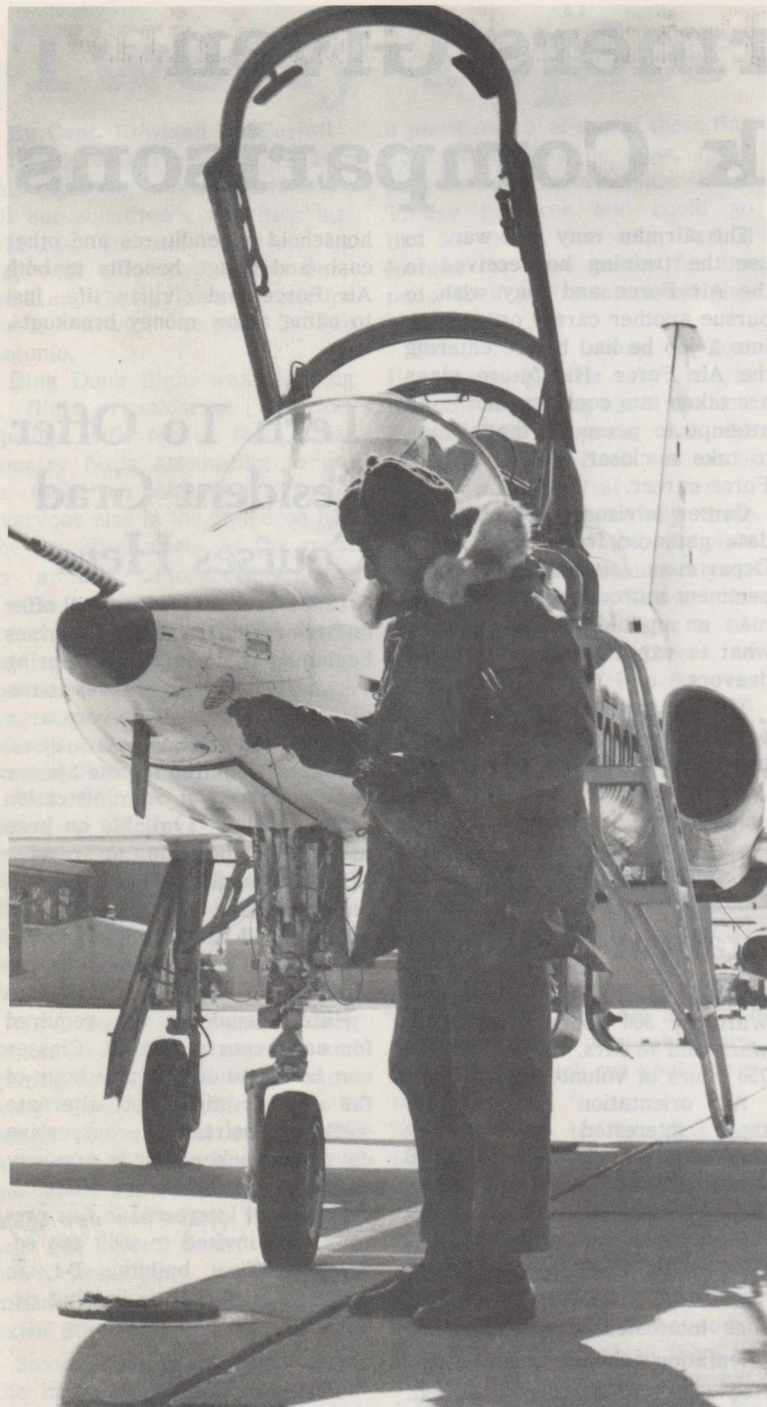
HOME AGAIN—SSgt. Roy R. Berggren, 3500th Organizational Maintenance Squadron crew chief, prepares to ground a Northrop T-38 Talon during recovery operations following return of the aircraft from one of the 195 sorties flown by the 3500th PTS Saturday. (Photo By SSgt. Deal Toney)
