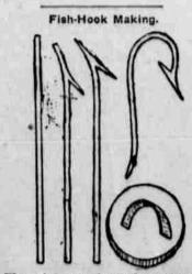
The pictures show the successive stages in manufacture of fish-hooks. The wire is cut in lengths and notched and bent while malleable.
