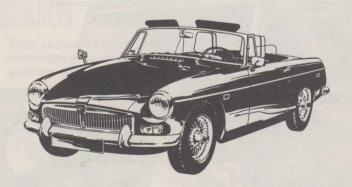
For performance: a 1798 c.c. twin-carb engine, fully synchronized four-speed gearbox, heavy-duty suspension, rack-and-pinion steering, and dual braking system with disc brakes up front.
