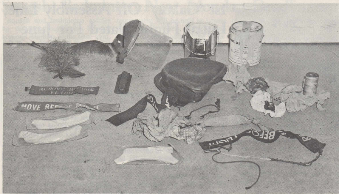
LOST AND FOUND—Just a sample of objects "lost" on the Reese flight line but found before they could cause engine damage. (AIR FORCE PHOTO)
