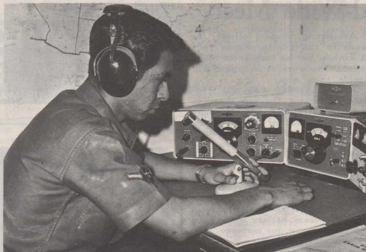
RECEIVES MESSAGE—A3C Richard Soltero receives a message over the KWM2-A transceiver at the MARS station. The transceiver is a combination receiving and transmitting set.
