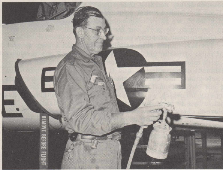
NEW PAINT JOB—Lee R. Smith puts the finishing touches of paint on the wing of a T-38 aircraft at Reese. The field maintenance squadron is conducting the work.
