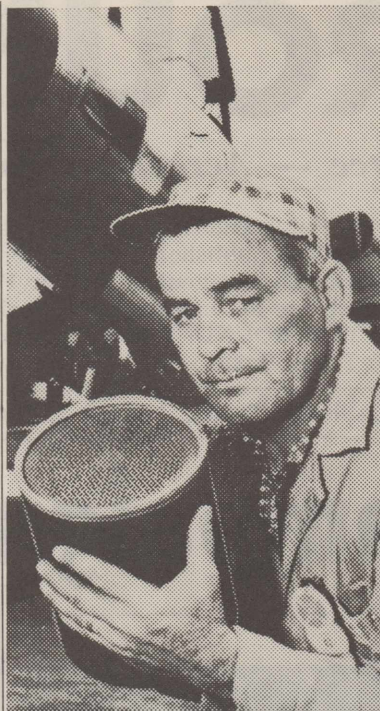
JET STARTER —The long, cylinder-like object held by a mechanic is a cartridge used to start the F-105D fighter-bomber in the background. A solid-propellant type starter, it enables the jet to be airborne in seconds.
