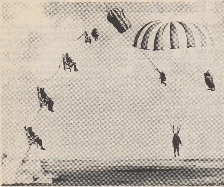
OVER AND OUT —Ejection seats were unheard of 50 years ago. But here pilot and seat are literally shot into the air in a test of a new rocket catapult seat-ejection system developed for the F-105D fighter-bomber. In this sequence-camera composite photo, starting at lower left: ejection begins with an explosive cartridge blast; the rocket ignites to lift the seat to 200 feet, where the pilot leaves it to parachute to earth; the seat, far right, hurtles on at a greater speed. The boost is designed to make ejection safer at low altitudes and during take-offs.
