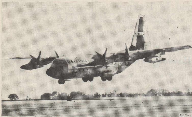
AIR BRAKES — A Lockheed Hercules C-130 eases down into an extra-short landing in a demonstration at Dobbins AFB near Atlanta. The huge transport, equipped with a Boundary Layer Control system prevents stalls at slow speeds, can land in less than 4½ times its own length—a shorter distance than the landing space required by a small, single-engine plane.
