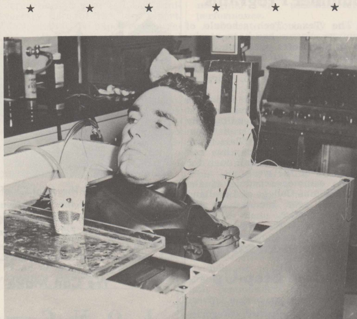
MAN IN A SPACE TUB —Capt. Duane Graveline lived seven days in a spaceage bathtub during an experiment at Air Training Commander's School of Aviation Medicine. While in the tub, the Air Force flight surgeon took his specially prepared liquid diet through a straw. The experiment was to determine what effects prolonged floating—at a state in many ways similar to weightlessness of Aerospace flight—has on the human body.
