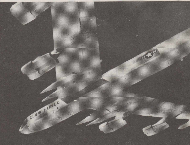
FLYING MISSILE LAUNCHER — This underside view of an Air Force B-52H global bomber, shows off to advantage its new armament. The marriage of manned bombers and hypersonic missiles provides an elusive aerial missile pad, with mobility from tree-top to 60,000 feet plus a striking range of thousands of miles.
