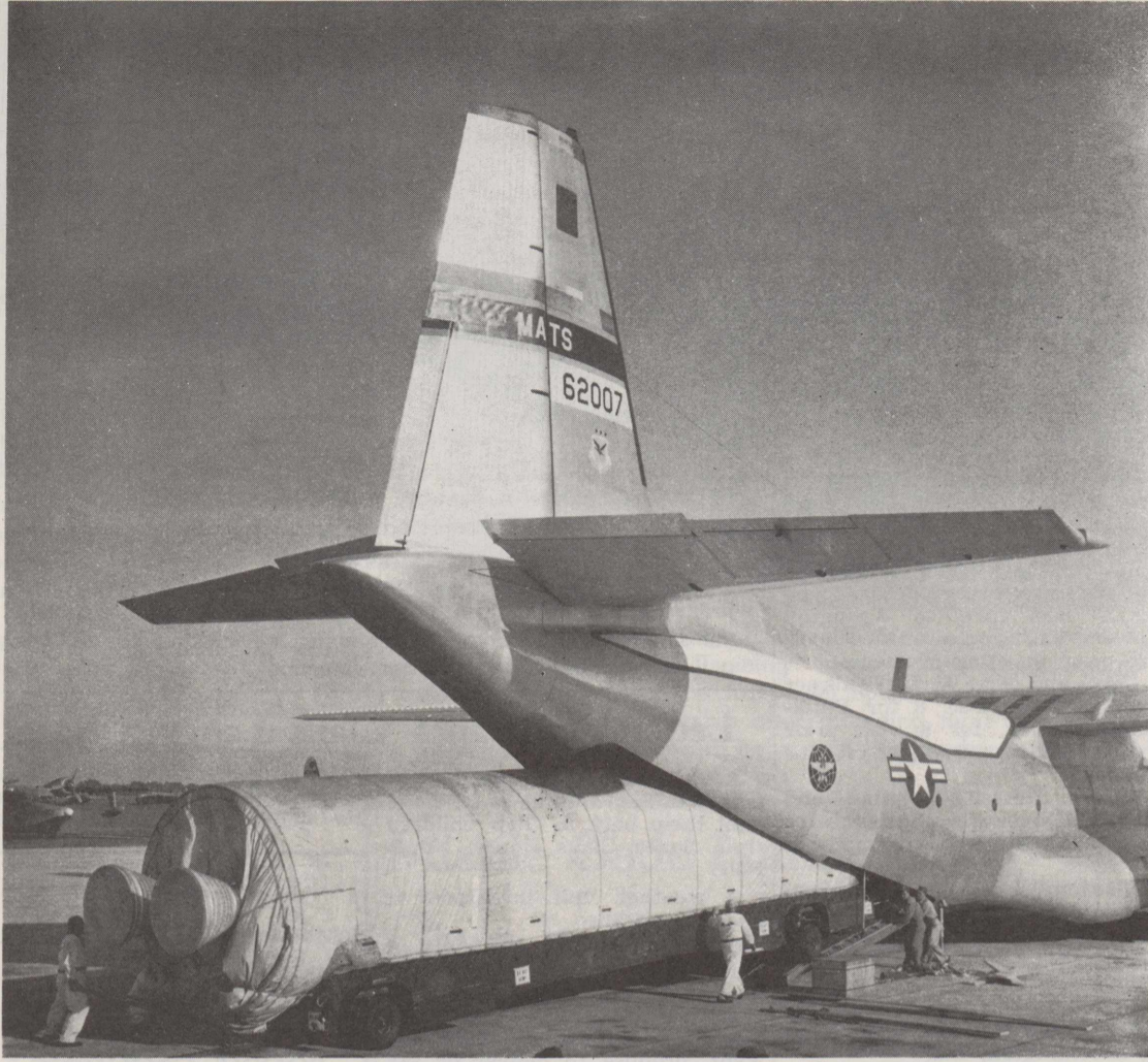
GIANT MEETS GIANT. The second stage of the 5,000-mile Titan ICBM gets extra airlift mileage as it is fitted into the huge cargo hold of the Douglas C-133 Cargomaster.
