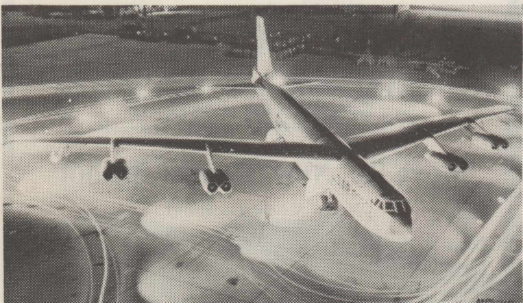
ON THE RAMP — This B-52 Stratofortress is on 24-hour alert training operations at Travis AFB, Calif. The jet bomber has an operational speed of more than 650 mph at altitudes higher than 50,000 feet. The single fueling range is 6,000 miles, but with in-flight refueling, only the crew's physical endurance limits the bomber's reach.
