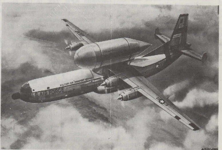
PIGGYBACK AIRLIFT—Artist's drawing shows an Air Force C-133 carrying the second stage of a Saturn C-1 missile in piggyback fashion. The method was proposed by the National Aeronautics and Space Administration to airlift the second stage from tests in Sacramento, Calif., to its launch site in Cape Canaveral, Fla., in only 10 hours. The original plan, requiring 24 days, called for shipment by barge.
