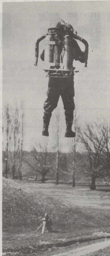
WINGLESS FLIGHT — A new man rocket controlled flight is demonstrated by the Army Transportation Research Command. The rocket, attached to the back, has flown man to the top of 30-foot hills and traveled ground distances up to 300 feet. It is powered by a twin-jet hydrogen peroxide propulsion system.
