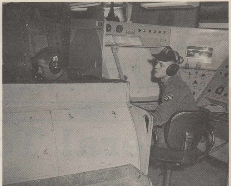
FLEDGLING—An aviation cadet training in a C-11 synthetic trainer is being observed by his instructor, AIC Donald Biderup. The trainer duplicates flight conditions of a T-33 aircraft.
