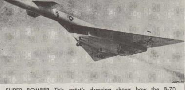
SUPER BOMBER-This artist's drawing shows how the B-70 Valkyrie bomber, slated for flight testing later this year, will look on take-off. It will be capable of flying at 2,000 mph, using six jet engines. Its predecessor, the B-52 Superfortress, has eight jet engines suspended from the wings. The Valkyrie represents departure from this design by housing its engines together underneath the fuselage. Flight tests on the first prototype will be conducted at Palmdale, Calif.
