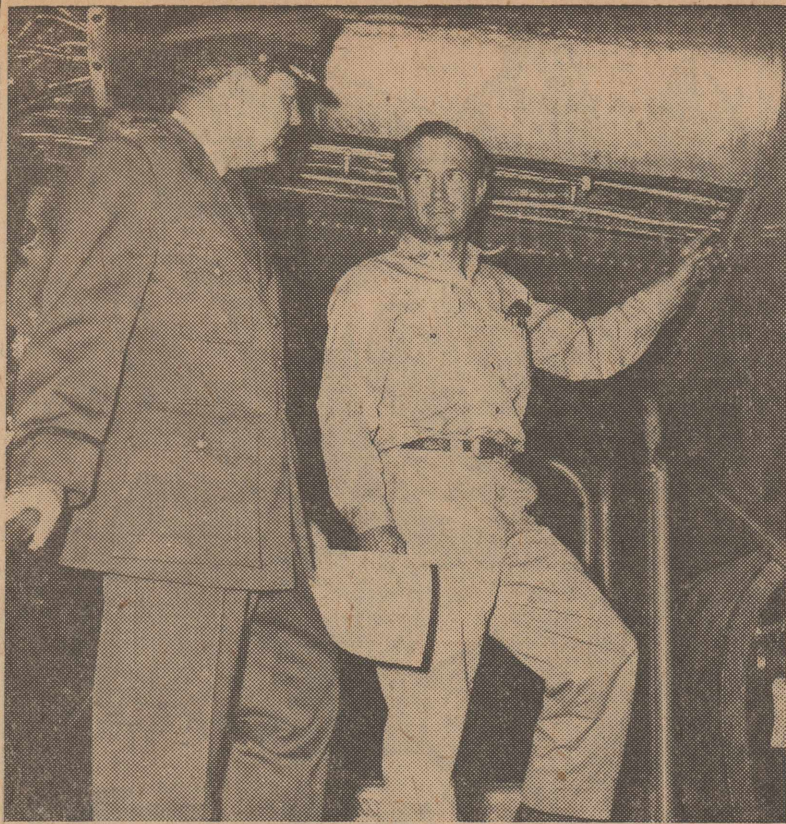
IMPROVEMENT SUGGESTION — Russell D. Townsend, 3505th Field Maintenance squadron shows the placement of reinforced doublers that secure the wing tunnel doors on the B-25 to Col. James C. Watkins, M&S group commander. His suggestion won a $75 award from the base incentive Awards Committee and the Air Material Command plans to include the idea in the Unsatisfactory Report Digest. (Photo by Haynes.)
