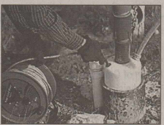
An E-Line is used to make a depth-to-water level measurement in an observation well located within the 16-county HPWD service area.
