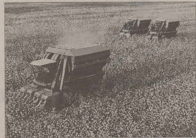
Courtesy Photo The 4-row cotton picker was introduced by John Deere in 1980 which increased operator's productivity by 85-95%.
