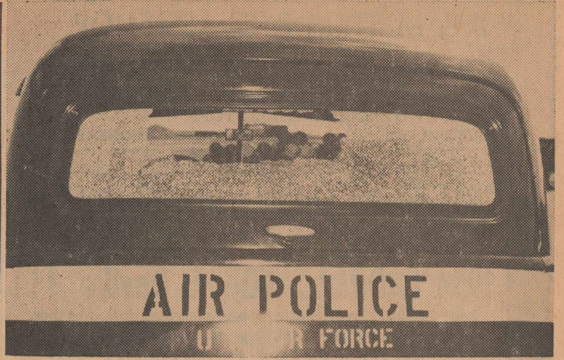
WHAT HAPPENED HERE? — No one seems to know what caused the glass to crack in this unusual pattern. What we do know is the glass is called Herculite and has been known to break at many different extremes of temperatures. Do you have any ideas? (Photo by Wilhite, Base Photo Lab.)
