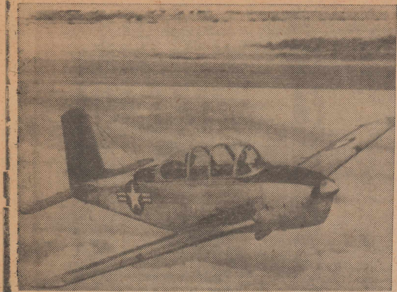
NEW TRAINER —The Beechcraft T-34, presently in production as an Air Force trainer, has been recently selected as the new Navy primary trainer. The two-place aircraft is powered by a 225 horsepower engine and has a top speed of 189 miles per hour. Gross takeoff weight is about 2900 pounds, and the all metal plane has a fully retractable tricycle landing gear. Air Force plans are for the T-34 to gradually replace the T-28.
