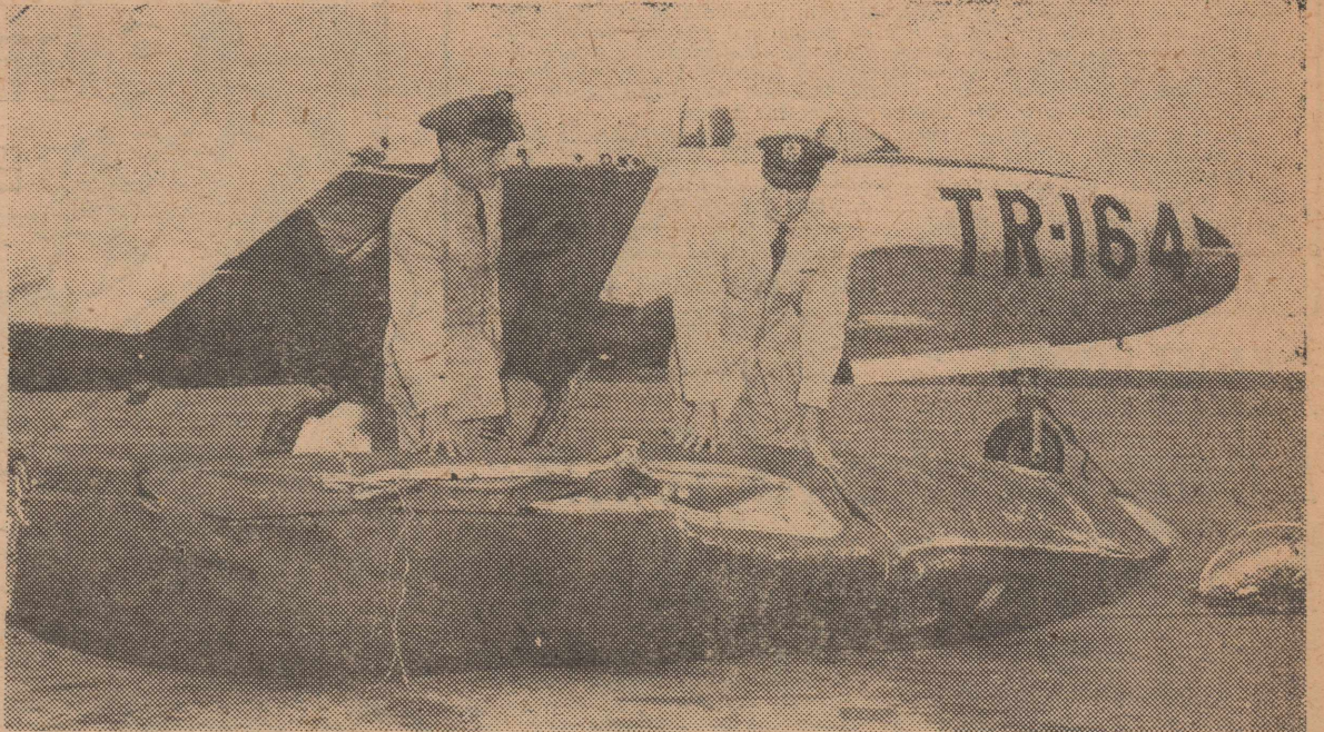
LETHAL—2nd Lt. Charles L. Jones, left, and 1st Lt. Vernon L. Wright, both stationed at Nellis AFB, Nev., inspect a battered wing tank that was wrenched from their T-33 jet trainer during a local storm. The tank fell to earth in the middle of Slaton, but luckily caused no damage.
