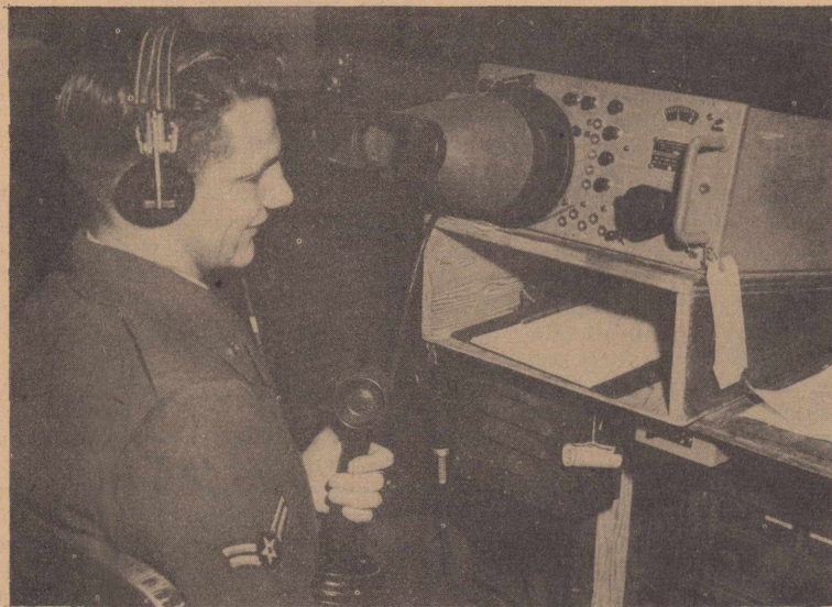
BRINGING HOME the lost ones with the aid of a new VHF direction finding unit is A-2C Don Welsko, DF operator. Recently installed in the control tower at Reese, the unit will assist aircraft that are lost in dust and foul weather.
